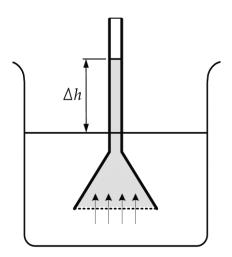
We will try to carry out a classical experiment on demonstration of osmosis. The principle is shown in the figure. Water moves from the solution of lower osmolality, across the semipermeable membrane, into the solution of higher osmolality, and its level rises. In theory, the process should stop in time of balancing the osmotic pressure by hydrostatic pressure of the column of the solution inside a tube.
