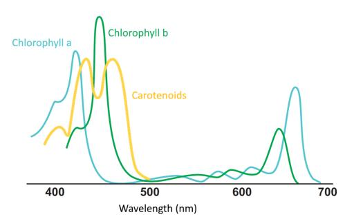
If we monitor which wavelengths a certain dye absorbs, we obtain the so-called *absorption spectrum*. This spectrum shows maxima (so-called peaks), which are typical for a given substance. It is ideal to monitor the absorption spectrum in the visible region, which is sufficient to identify several dyes contained in the leaves. Decomposition products of chlorophyll are pheophytins, carotenoids pass through epoxides to colorless compounds.
