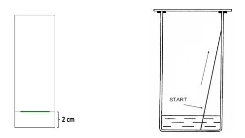
Draw the base-line about 2 cm from the shorter edge of the plate. Use the thin pencil. Do not press on the pencil to tear of the sorbent layer!
