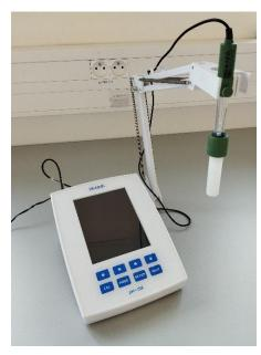
There is a pH meter with combined electrode (consisting of both the glass and the reference electrode) at your working place.
