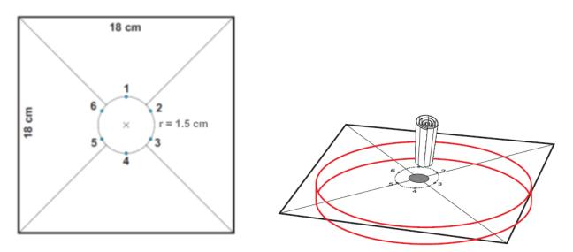
Place the paper into a Petri dish partly filled with a solvent mixture (n-butanol, acetic acid, water -4:1:1) and cover the paper with a cap.
