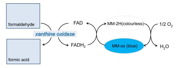
This experiment can be used as a simple test for milk pasteurisation. Higher temperature causes enzyme denaturation and adding of formaldehyde cannot raise discolouration of methylen blue.
