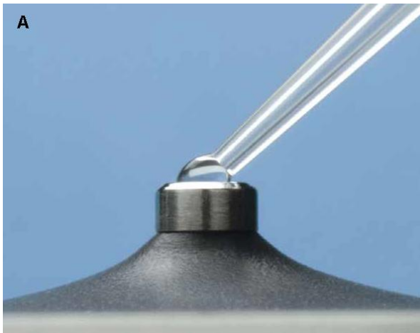
Pipetting sample solution onto pedestal
